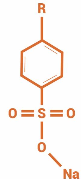
Schematic illustration of Mono Alkylbenzene Sodium Sulfonate.
